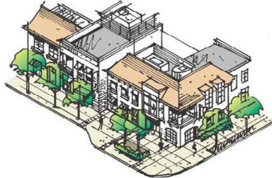
Example of screening equipment with roof forms.
